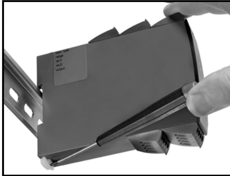
Picture 1: Detach the module from the DIN rail by lifting the bottom lock.
